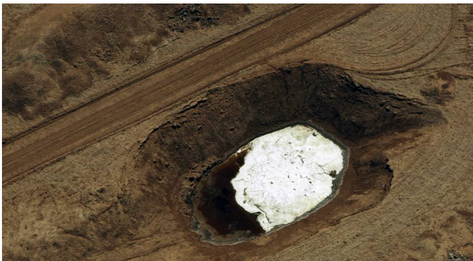
Figure 6. Oblique air photo captured on August 23, 2011 to estimate angle of pit wall and confirm water table.
