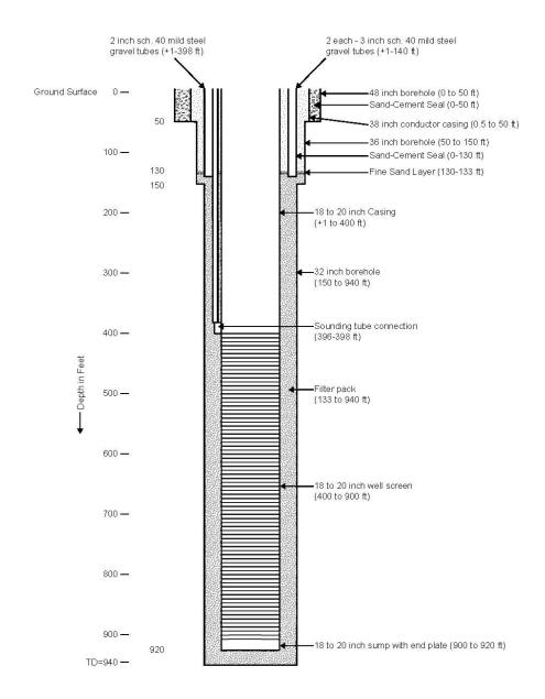
FIGURE 5-4 Conceptual Well Design Diagram
