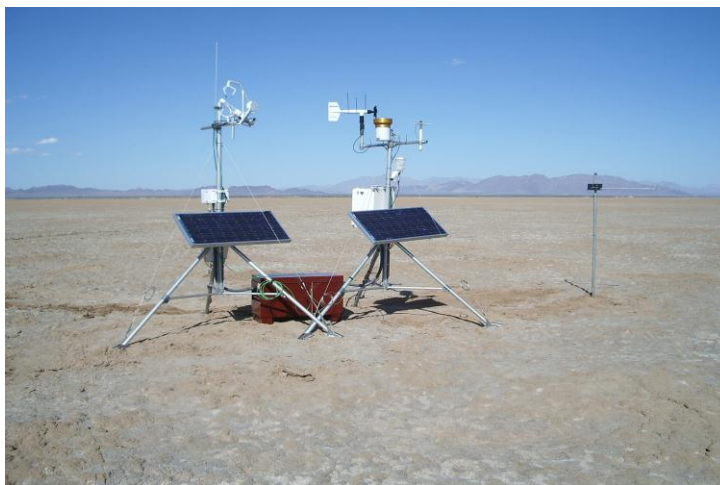
Figure 1. Eddy covariance (EC) and meteorological towers and instrumentation located on Bristol Dry Lake located near Cadiz, California.
